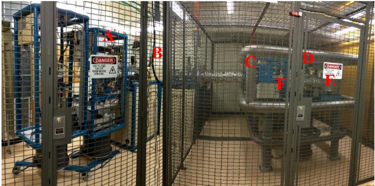
Fig. 3: Different views of two accelerator mass spectrometers (AMS). Top (ANSTO): A = the ion source; B = the injector magnet; C = the tandem accelerator; D = the analysing magnet; E = the electrostatic analyser; F = the gas ionization detector (Image: ANSTO); Bottom (single stage accelerator mass spectrometer at ANU). A = the iron source; B = the injector magnet; C = the high voltage deck accelerator; D = the analysing and switching magnet; E = the electrostatic analyser; F = the silicon barrier detector (Image: ANU).
